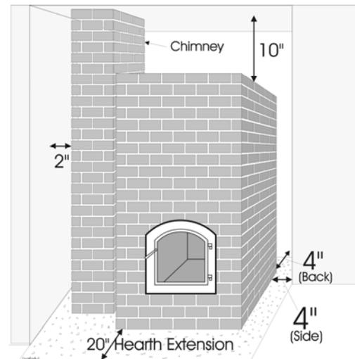
NOTE: a combustible wall with non-combustible material applied directly to it without an intervening air space *IS STILL A COMBUSTIBLE WALL FOR PURPOSES OF CLEARANCES*. If clearances must be reduced, a simple method is to build a wall behind the fireplace, in the area of concern, constructed of "cement board" (a 1/2" [12.5mm] cement sheet) installed on metal studs. This wall section must extend 8" (200mm) beyond the sides of the fireplace.
