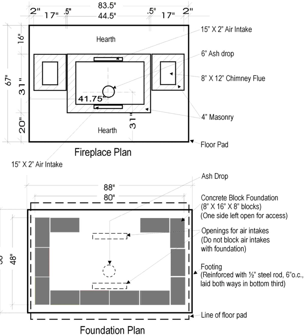
**NOTE:** If back-up block is required around the chimney, (eg. for stone facings), footing, foundation and pad dimensions will require suitable adjustment.
