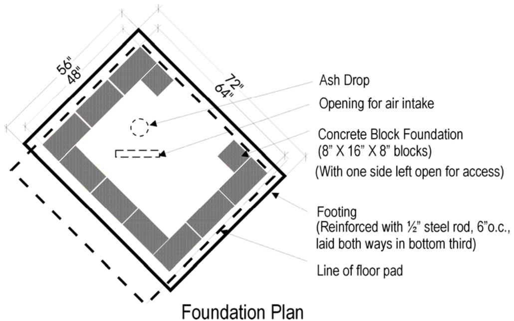
**NOTE: If back-up block is required around the chimney, (eg. for stone facings), footing, foundation and pad dimensions will require suitable adjustment.**
