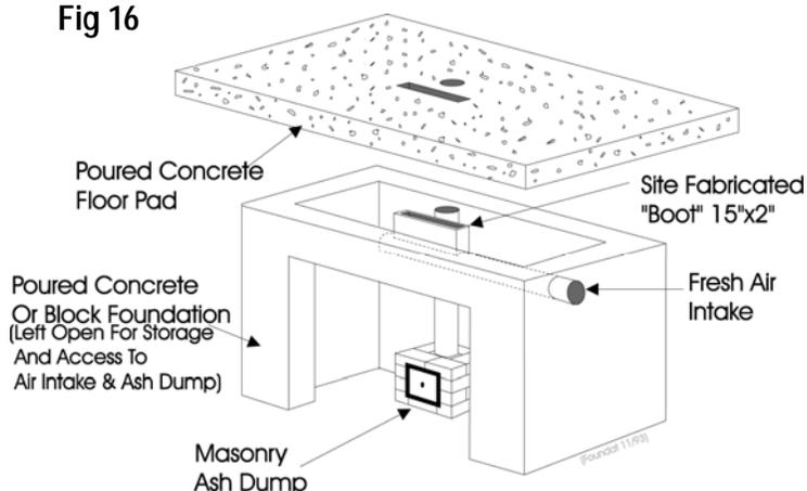
smooth duct is built into the top course of foundation blocks, which will feed necessary air into a 15" x 2" (380mm x 50mm) hole located in the floor pad, directly in front of the unfinished core. The duct is vented to the outside wall under the floor joists and can be equipped with an optional electrically operated damper.
