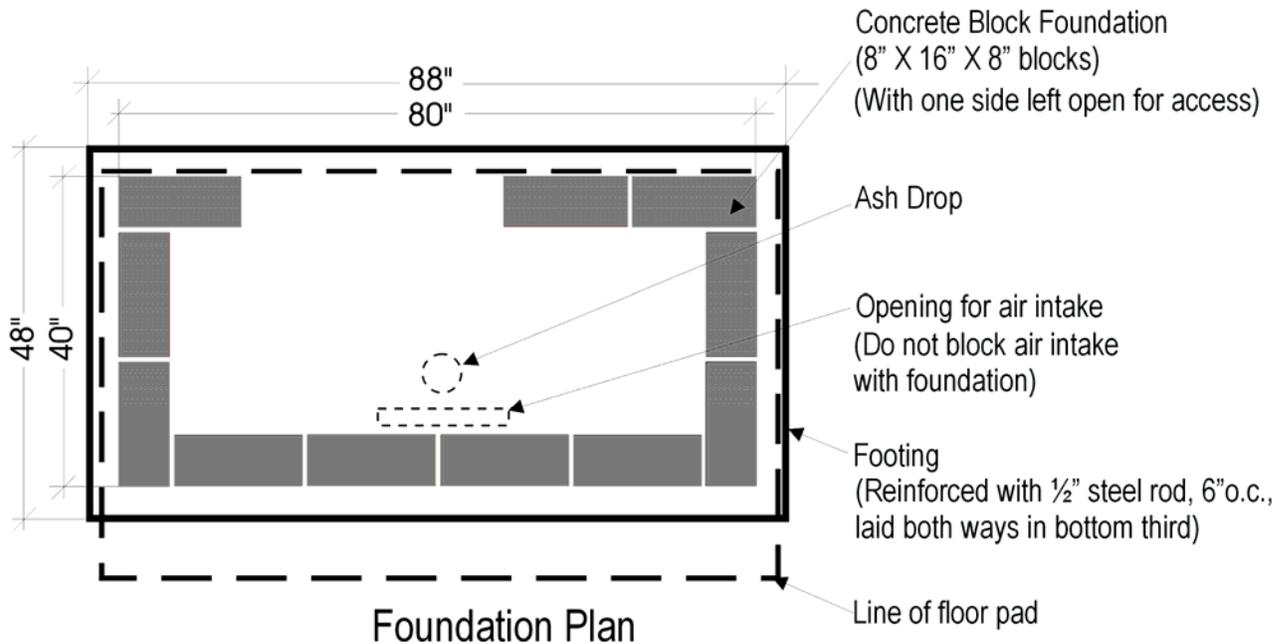
**NOTE: If back-up block is required around the chimney, (eg. for stone facings), footing, foundation and pad dimensions will require suitable adjustment.**
