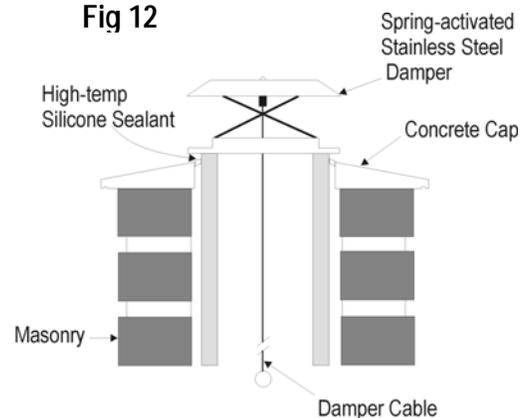
The 'hybrid' chimney combination is possible *only where the chimney is straight*, (ie. without any offsets) so that the cable is not obstructed. If there are offsets in the chimney, then we recommend installing a Base-exit Transition, with internal damper, and either an approved (i.e."listed") stainless steel liner and masonry chimney facing or a full factory-built chimney system. (*An adapter on top of the transition, manufactured for the chimney being used, will be required.*)
